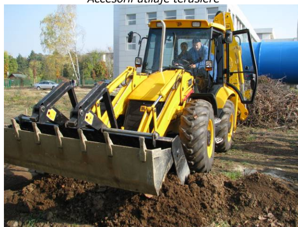
Buldoexcavator JCB 3CX – lucrări practice
