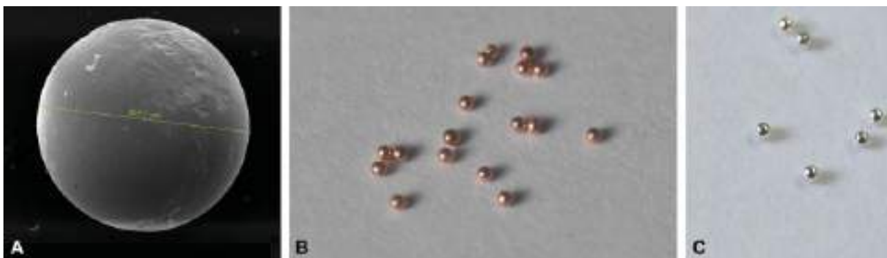
Fig. 1 Scanning electron microscopy image of a copper particle (A). Photographic images of copper (B) and silver (C) spherical particles.
