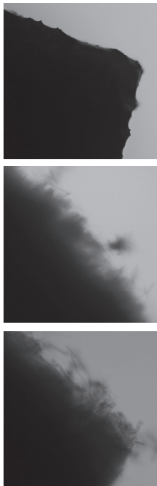
Photo 3. Microscopic aspects of bovine pelts incubated for 10 days with the bacterial isolate BN7 (middle and down) comparative with the untreated sample (up)
